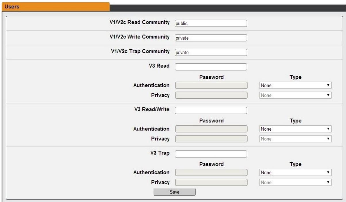
The image shows the Users configuration page. It contains three sections for V1/V2c and V3 configurations. Each section has a "Community" or "Trap" field, a "Password" field, and "Authentication" and "Privacy" dropdown menus. The "Authentication" and "Privacy" dropdowns are currently set to "None". A "Save" button is located at the bottom of the page.
